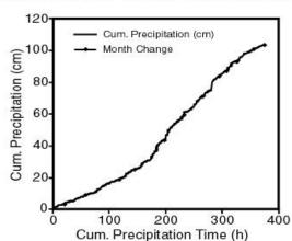
Figure 5. Cumulative precipitation vs. cumulative precipitation time for one year.
