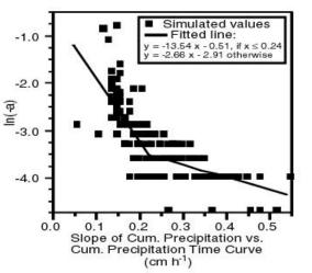
Figure 6. Approximating coefficient "a" from the slope of cum. precipitation vs. cum.
