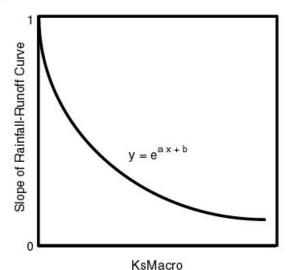
Figure 3. Slope of rainfall-runoff curve vs. KsMacro
