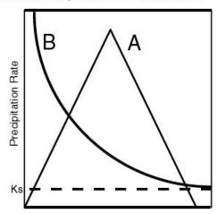
Figure 1. The time-to-ponding approach to infiltration. Curve A is the precipitation rate vs. cumulative precipitation. Curve B is the precipitation rate above which water ponds. Ks is the matrix saturated hydraulic conductivity of the top layer.
