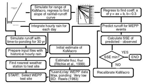
Figure 7. Calibration with WEPP Hillslope Data Sets: Method.
